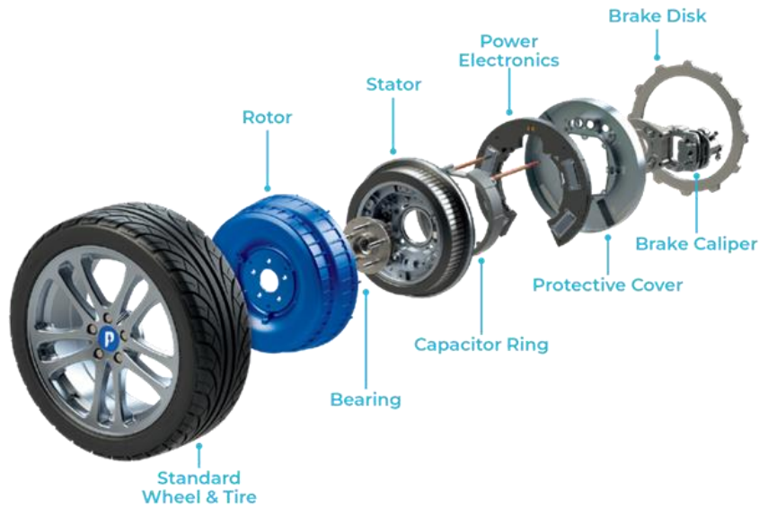
Figure 7.12 The components of an in-wheel electric motor. The PD18 incorporates the power electronics and a disc brake to replace the OEM brake, making the packaging exercise much simpler [25].
