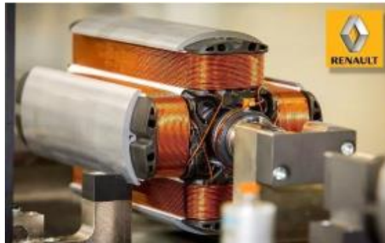
Figure 7.10 A rotor with windings connected to slip rings on wound-rotor synchronous motor [20].
