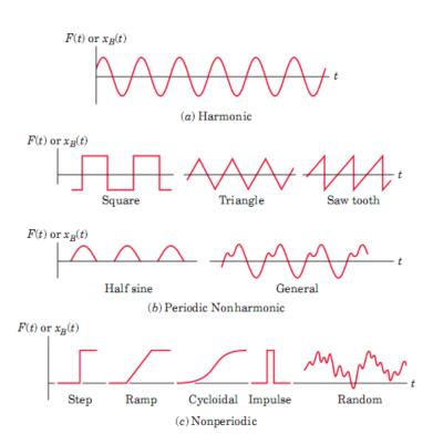
If there is present some disturbance force that impacts on free harmonic vibration motion, then that motion is called FORCED VIBRATION.
