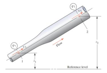
The amount of fluid that passes through any crosssection at any point in time is constant.
