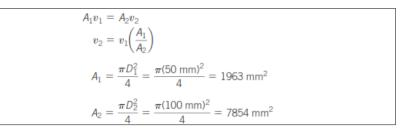
$$v_2 = v_1 \left(\frac{A_1}{A_2}\right) = \frac{8.0 \text{ m}}{\text{s}} \times \frac{1963 \text{ mm}^2}{7854 \text{ mm}^2} = 2.0 \text{ m/s}$$
