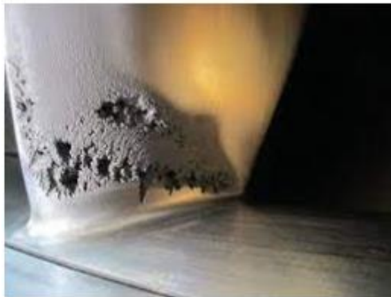
Fig. 14. Picture of actual cavitation damage runner [Chrisopher. 1994].
