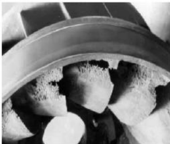
Fig. 14. Picture of actual cavitation damage runner [Chrisopher. 1994].
