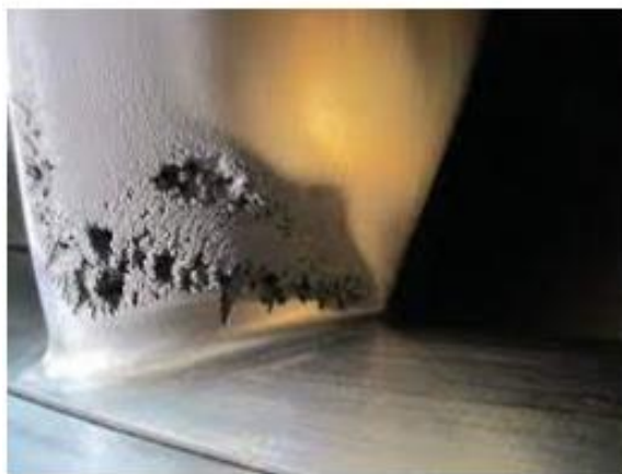
Fig. 14. Picture of actual cavitation damage runner [Chrisopher. 1994].
