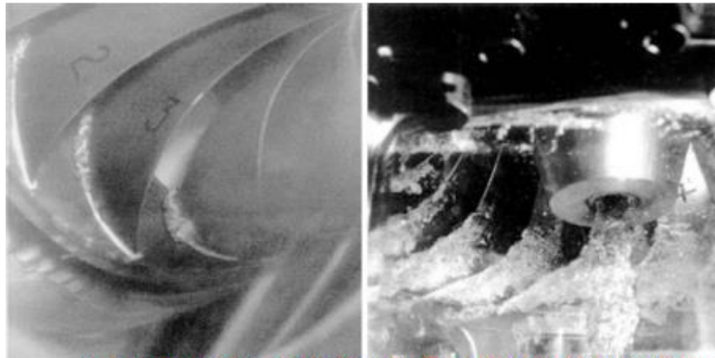
a. Leading-edge cavitation. b. Travelling bubble cavitation.
