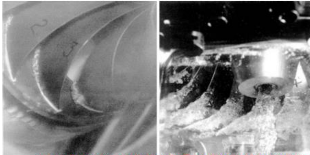
a. Leading-edge cavitation. b. Travelling bubble cavitation.
