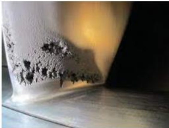
Fig. 14. Picture of actual cavitation damage runner [Chrisopher. 1994].
