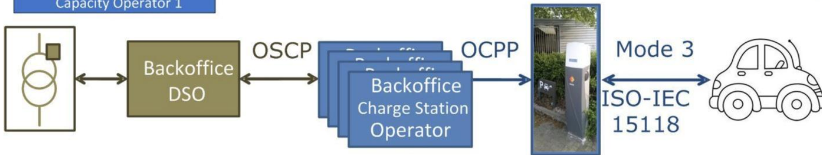
Fig 7: Depiction of the Open Smart Charging Protocol (OSCP)
