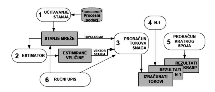
Structure and sequence of EMS calculation execution in the management of transmission networks.
