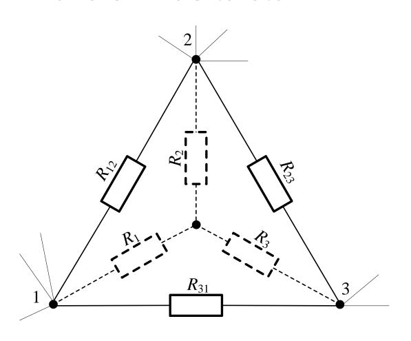
$$R_{1} = \frac{R_{31}R_{12}}{R_{12} + R_{23} + R_{31}}$$
