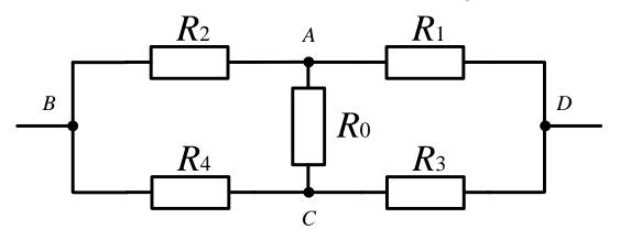
$$\begin{split} R_{24} &= R_2 + R_4 \quad R_{13} = R_1 + R_3 \\ \frac{1}{R_{AC}} &= \frac{1}{R_0} + \frac{1}{R_{13}} + \frac{1}{R_{24}} = \frac{1}{R_0} + \frac{1}{R_1 + R_3} + \frac{1}{R_2 + R_4} \end{split}$$
