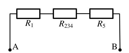
$$\frac{1}{R_{234}} = \frac{1}{R_2} + \frac{1}{R_3} + \frac{1}{R_4}$$
