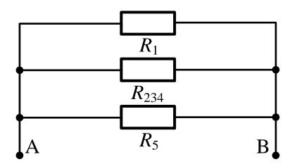
$$R_{234} = R_2 + R_3 + R_4$$
