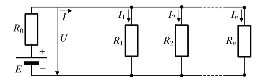
$$\frac{1}{R_{\text{ek}}} = \sum_{k=1}^{n} \frac{1}{R_k} = \frac{1}{R_1} + \frac{1}{R_2} + \dots + \frac{1}{R_n}$$
