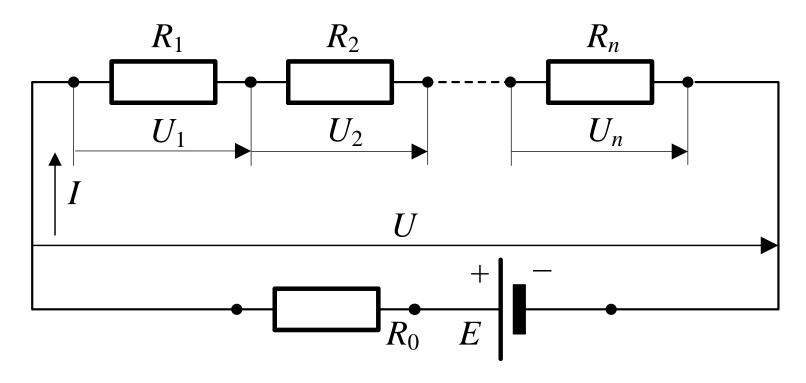
$$R_{\text{ek}} = \sum_{k=1}^{n} R_k = R_1 + R_2 + \dots + R_n$$
