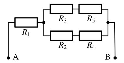
$$R_{24} = R_2 + R_4$$
